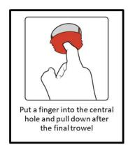
Pull the protector out slowly without twisting or damaging the plaster
